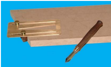
James Childress' Marking Knife made from steel, brass, and walnut. And a dovetail gauge made from Brass kick plate and a piece of iron-wood.
