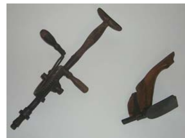
Don Kruse' small hand held Adz, and a Breast Drill with hand crank
