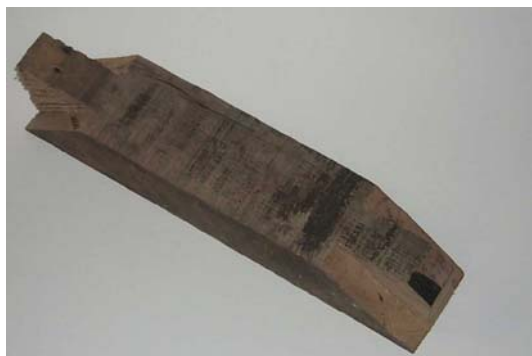
Ray grahams piece of wood for a gazebo, which required a mortise and tenon
